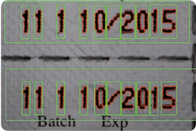
This application checks the variable data printed on the aluminium blisters by inkjet printers, after the blister sealing.
