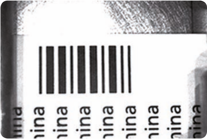
This is a comparison check between the printed code on the product and reference code inserted at production batch start. OCV supports linear pharmacodes, high density linear codes and 2D codes (Datamatrix).
