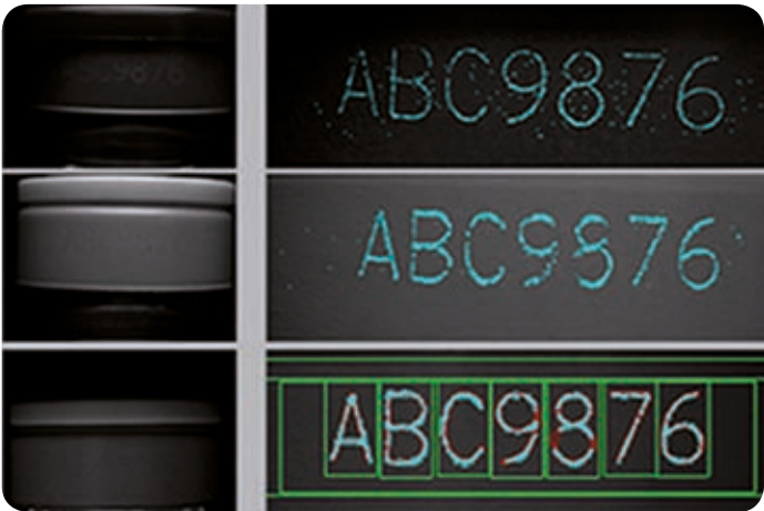
Check of laser-printed characters on vial's aluminium skirt.
