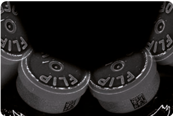
2D code check on the product's skirt. This 360° inspection is necessary due to the random positioning of the DataMatrix code on the skirt.
